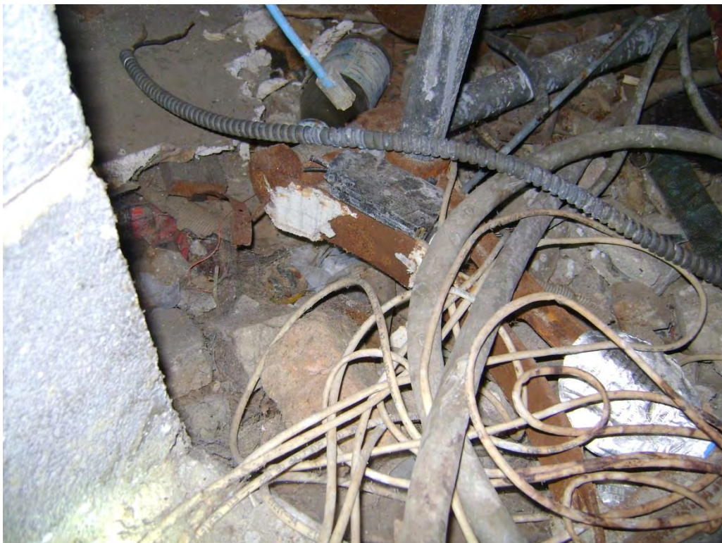
Sample #157 - Debris on Metal Support - 28.60% Chrysotile
