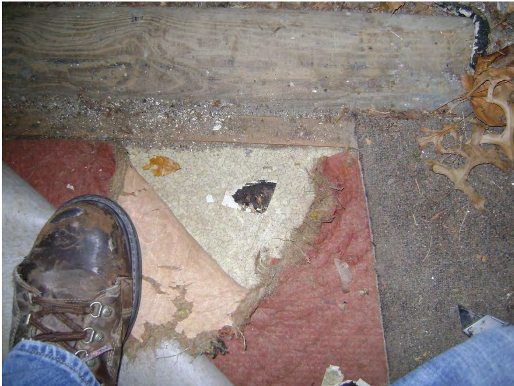
Sample #196 – Linoleum and Mastic – 11.4% Chrysotile
