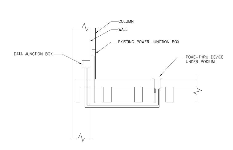
3 ELECTRICAL POKE-THRU DETAIL 3 SCALE: N/A
